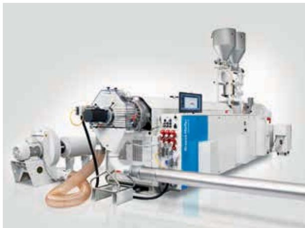
A twin-screw extruder for PVC pelletizing is used in production at Polymer Compound, Moscow, Russia.
