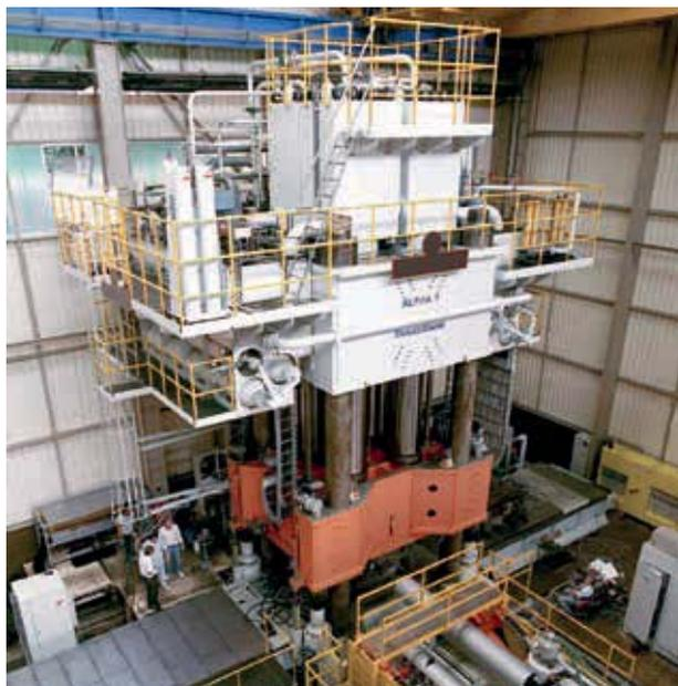
Legend: the Alpha 1, a multifunctional laboratory machine with a clamping force of 5,000 tons.
